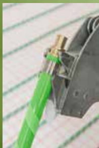
Production of a permanently fixed PRINETO sliding sleeve connection
